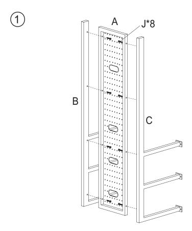
1-Attach frames (B) & (C) to the back panel (A) with screws (J).
